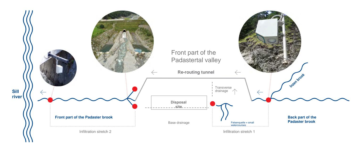
Different measuring stations (radar and measuring weir)
